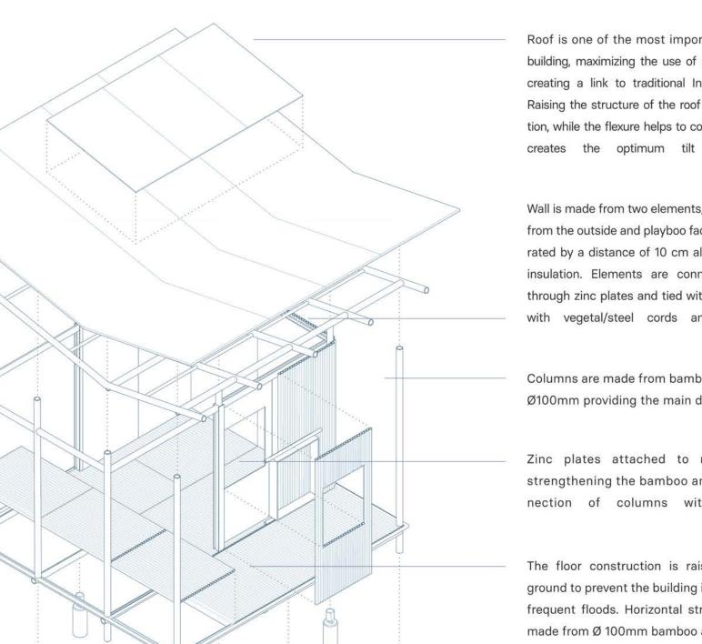
Roof is one of the most important elements in the building, maximizing the use of natural conditions and creating a link to traditional Indonesian architecture. Raising the structure of the roof allows natural ventilation, while the flexure helps to collect the rainwater and
