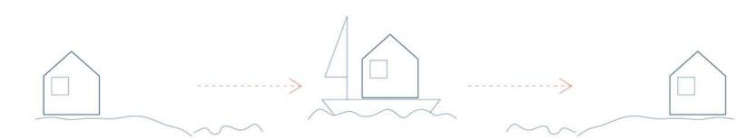
Due to the fact that Indonesia consists over 17 thousand islands and the refugees are spread across the whole country the house has to be portable. Therefore the elements of the structure don't exceed 1,7 x 5,5m and can be easily transported. The segments will be made in a workshops and when ready can be transported and connected on the spot in one day. With an aproxiamted weight of only 500 kilos per segment MAST can be placed wherever is necessary.
