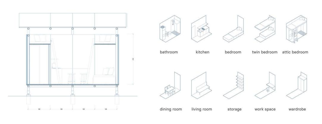
The interior of the house can be created depending on the needs. There are several modules to choose from. The interior is mainly made of bamboo. The furniture in the modules can be produced by the inhabitants of the island in local workshops. The terrace is an additional space that can be a dining room, a living room or a place to relax.
