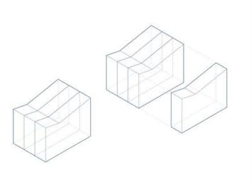
By creating modular, transformable spaces we want the house to react to the changing needs of building occupants. MAST is made from 1.2 meter wide segments, that can easily be connected and disconnected, to make the house highly flexible. Moreover, the segments can be reused over and over again and are recyclable.
