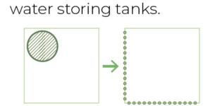
Tubes can be used as a permeable nonbearing wall that permits
